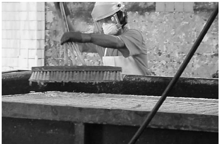
Figure 7—After immersion and impregnation, worker “brushes” asbestos diaphragm surface in order to smooth it, wearing an improper respirator.
